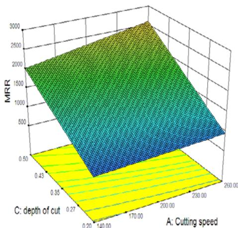
Fig 4.5 (b) 3D Surface graphs for material removal rate b/w depth of cut and speed
