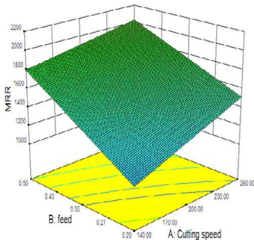
Fig 4.5 (a) 3D Surface graphs for material removal rate b/w feed and speed
