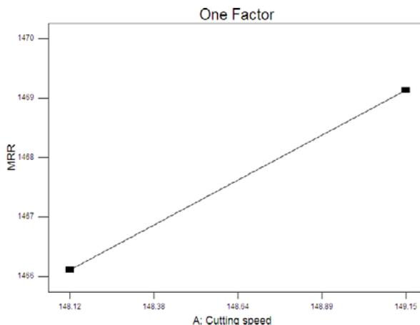
Fig. 4.4 (a) Effect of cutting speed on Material removal rate at constant feed 0.35 mm/rev and constant depth of cut 0.35mm
