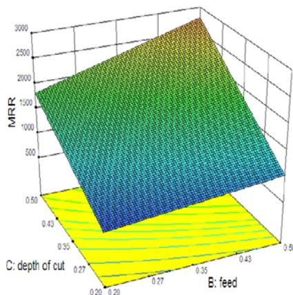
Fig 4.5 (c) 3D Surface graphs for material removal rate b/w depth of cut and feed
