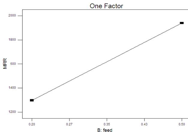
Fig. 4.4 (b) Effect of feed on material removal rate at constant cutting speed 200 m/min and constant depth of cut 0.35mm
