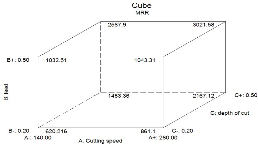
Fig. 4.6 Cube plot for material removal rate
