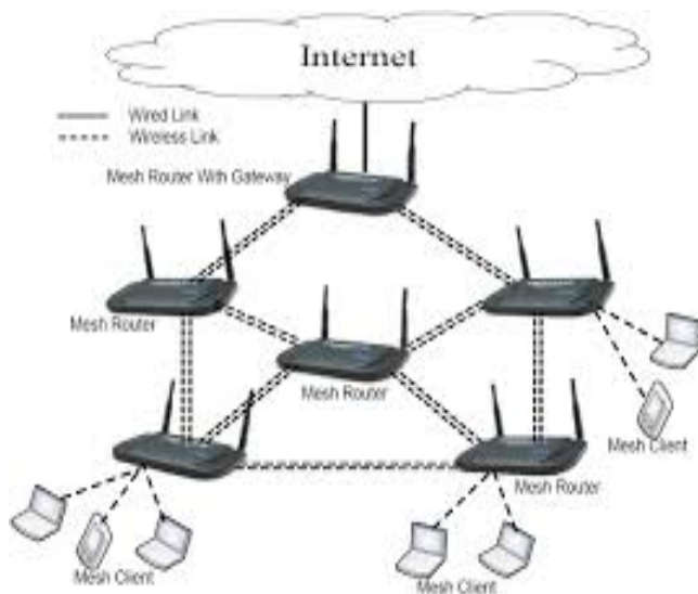
Figure 1: Network Architecture of wireless mesh network
