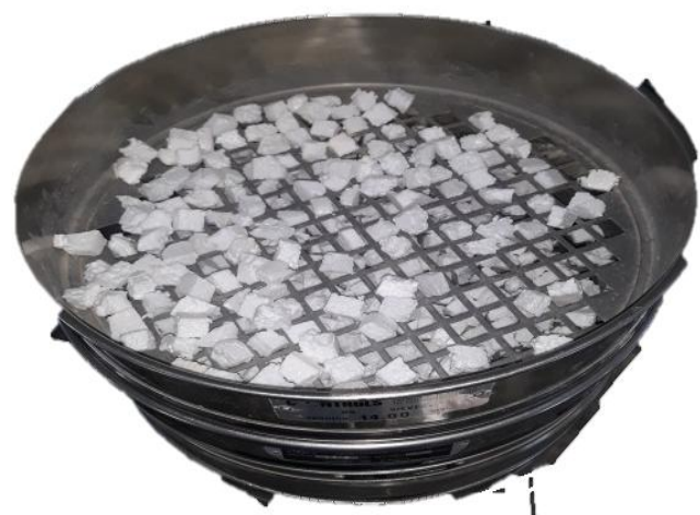
Figure 3: Sieve analysis of recycled Styrobar (EPS) particles
