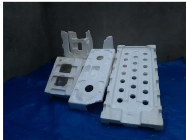
Figure 2: Recycled Styrobar (EPS) used in concrete mixtures
