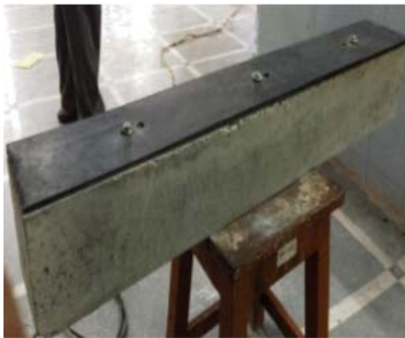
RCC Beam retrofitted with MS plates
