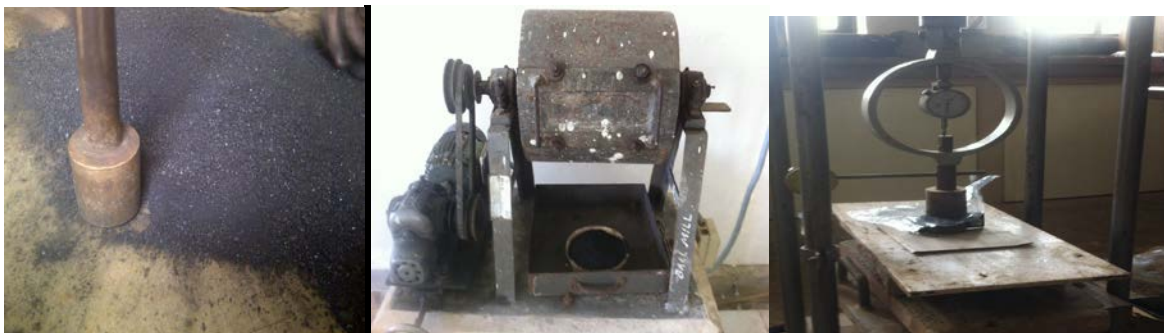
Figure 3: Crushing using ball mill and Mechanical Press applied on briquette
