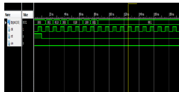
Figure 18: TPG using Graycounter, decoder and accumulator
