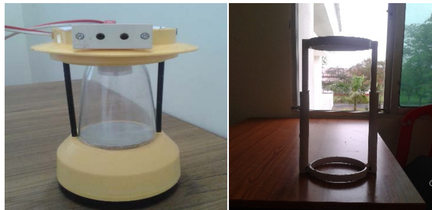
Fig 3.3: Closed and open holder (novel) design of solar lantern
