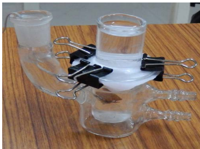
Fig.7 Bio-membrane and Franz Cell.
