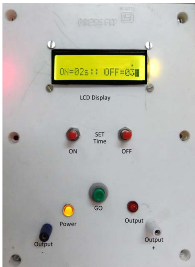
Fig 4 shows front panel of power supply
