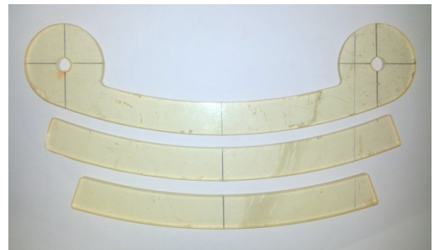
Fig. 4.2 Photo Elastic Model of Leaf Spring Having 20mm Leaves Thickness
