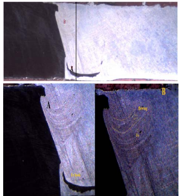
Fig 6: microstructure of parameter (Rotation speed 800rpm, tool offset -1mm, and travel speed 12mm/min)
