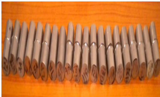
Figure 3.5: AISI 316 L stainless specimen after turning operation
