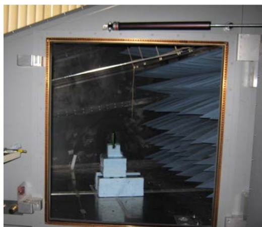
Fig. 3 The mobile station under test in the x- axis position in the GTEM. (GGIEMR, Nottingham University)
