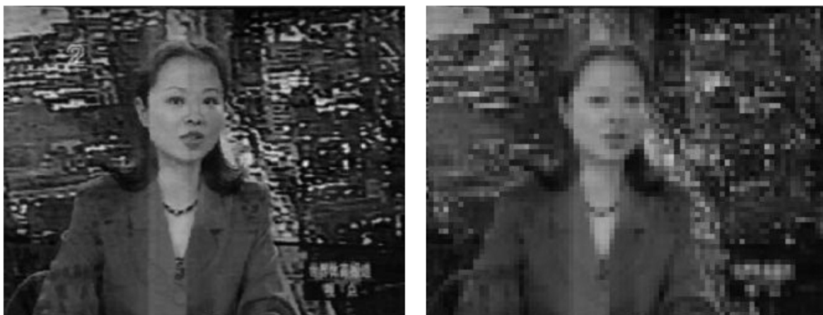
Figure 4: (a) Original image (320x240 pixels, face area: 44x48 pixels) b) Mosaic image (unit size=4x4 pixels)
