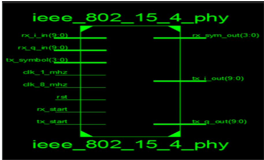
Figure 3: RTL schematic of Zigbee Transceiver
