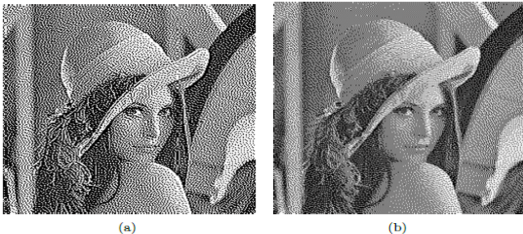
Figure 7: Half toning image by error diffusion. (a) The error diffusion weight matrix in Figure 6 (a) is used. (b) The error diffusion weight matrix in Figure 6 (b) is used.
