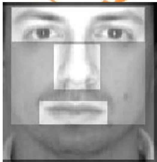
Figure 11: Whole face, eyes, nose and mouth regions that could be used in a template matching approach
